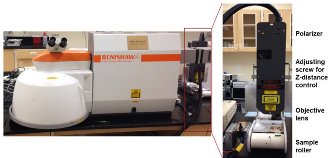
Fig. 9. Renishaw inVia micro-Raman system with custom-designed remote optical probe and roller sample stage.
