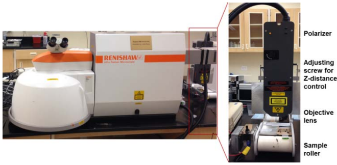
Fig. 6. Renishaw inVia micro-Raman system with custom-designed remote optical probe and roller sample stage.
